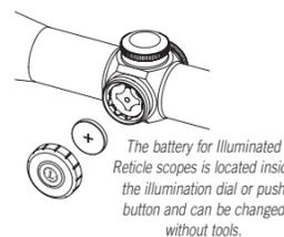
The battery for Illuminated Reticle scopes is located inside the illumination dial or push button and can be changed without tools.
